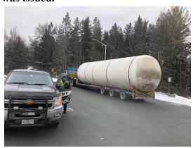
• 1/13 Lyndonville detail. An Inspector conducting a Level 2 inspection on a flatbed CMV placed the CMV out of service for improper load securement. Web
