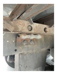
• 7/14 Inspector located severely corroded spring hangers on a trailer during an inspection at the Guilford Detail. Due to the axle not shifting from its normal position the violation did not meet the out of service criteria.
