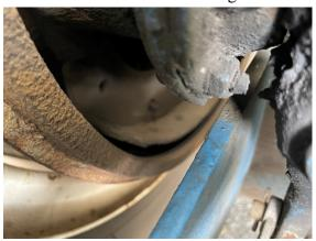
• 7/14 Inspector discovered a kinked air brake line during a level 1 inspection at the Guilford truck Check Detail.
