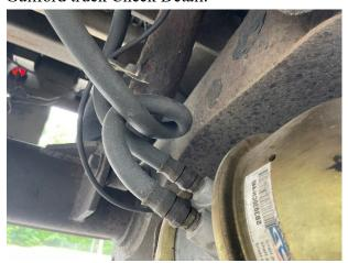
• 7/14 Inspector located a loose air reservoir tank and a crack in the cross member above the suspension of a trailer during a level 1 inspection at the Guilford Truck Check Detail. The vehicle was placed out of service.
