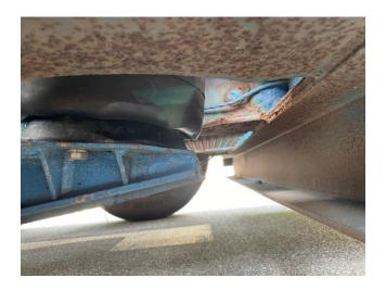
• 7/14 Inspector located a brake shoe with a missing lining during a level 1 inspection at the Guilford Truck Check Detail. Three additional brakes were also out of adjustment and the vehicle was placed out of service for more than 20% of the brakes on the combination being defective.
