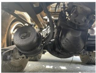
• 7/13 Inspector discovered a plastic service airline that was chaffed through the outer core, indicated by a color change in the hose. The trailer was placed out of service.
