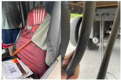
• 7/14 Inspector discovered a crack in the cross member of a van-type box trailer. The damage did not extend into the adjacent cross members and was noted as a defect only.
