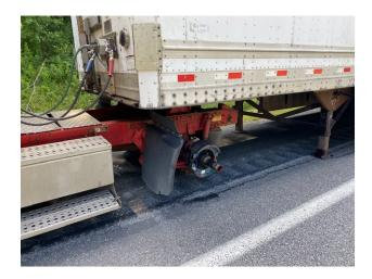
• 7/13 Inspector discovered a significant engine oil leak originating from several locations during a level 1 inspection at the WRJ detail. The oil contamination was so significant it covered most of the brake canisters and parts of the tire. The driver was warned that once the contamination extended onto the wheel surface or braking surface it would render the truck out of service.
