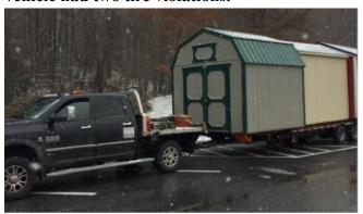
• 11/3 Inspector inspected an intrastate tractor trailer hauling machinery at the Ferrisburgh detail. One of the chains had no binder and had come loose in transit. This was a required tiedown, placing the trailer out of service until corrected.
