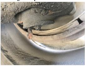
• 10/8 Inspector conducted a level 1 inspection at the VT Rte 9 Chain Up Area. Four brakes on the tractor trailer combination were out of adjustment. The vehicle was placed out of service and repairs were made onsite.
