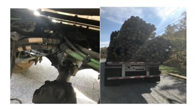
• 10/8 Inspector completed a level 1 inspection at the Bennington chain up area on a truck towing a modular home. Both rear lower brake linings on the truck had small cracks. Four of the trailer wheel seals were leaking and oil/ grease had contaminated the braking surface. In addition, one of the trailer hub caps was missing. The carrier was issued a ticket.
