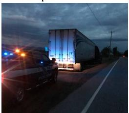
• 10/6 Inspector, at the Fair Haven detail, inspected an interstate tractor trailer. The trailer was placed out of service for inoperable turn signals.
