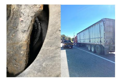
• 10/7 Inspector discovered a gouge in the side wall of a tire while conducting a level 2 inspection at the Hartford detail. The damage was found to extend into the plies.
