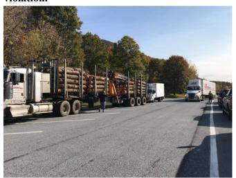
• 10/15 Inspector inspected a tractor trailer at the Ira detail. A subsequent inspection revealed the brake lights were inoperative on the trailer, four out of ten brakes were defective and the frame on the trailer was cracked. Both the combination and the trailer were placed out of service. The carrier was ticketed.
