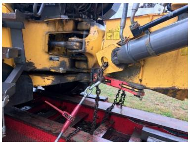
• 10/13 Inspector inspected a tractor trailer at the Colchester detail. The CMV was placed out of service for not displaying oversize banners as required and for loose chains over the equipment.
