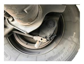
• 10/12 Inspector discovered a tire with a bulge due to sidewall separation during an inspection at the Putney Scale House. The vehicle was placed out of service and the tire ruptured during the inspection.
