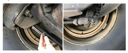
10/14 Inspector completed a Level 1 inspection of a 5-axle combination vehicle and found multiple cracks in the brake linings and a separation from the brake shoe. The vehicle was placed out of service until repaired.
