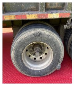
• 10/13 Inspector discovered several brakes out of adjustment while conducting a Level 1 inspection at the Bridgewater detail. The CMV was put out of service for the 20% brake criteria. At the time of the inspection the brake was inoperable, and the brake liner did not touch the brake drum.
