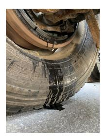
• 10/12 Coventry Village detail. An Inspector conducting a Level 1 inspection on a six axle CMV placed the CMV out of service for defective brakes- greater than 20% of the brakes were defective.
