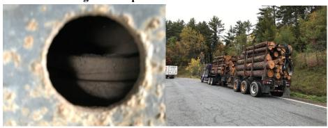
• 10/14 Waterford detail. An Inspector placed a five axle CMV out of service in combination after a trailer brake supply hose was found to be defective. A ticket was issued to the carrier.
