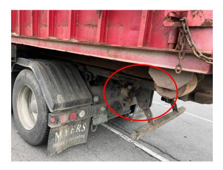
• 5/10 Insp. inspected a tractor trailer on Rte. 22a in Shoreham. The trailer was placed out of service for a leaking hub.
