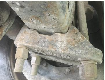
On 05/11 Insp. discovered an oil leak during an inspection at the Emerald Lake detail. The leak was from a cracked repair weld on the axle housing. This defect is a violation only and did not put the vehicle out of service.
