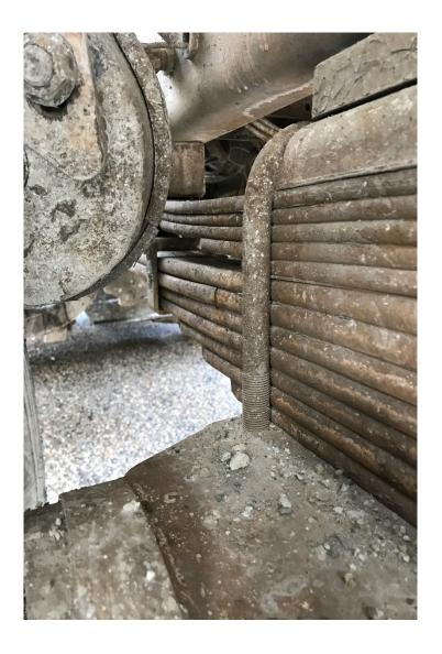
• 12/10 Inspector placed a CMV out of service for a deflated tire. The inner tire was deflated to 20 PSI and was rubbing on its mate in a dual set.
